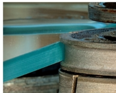
Edge grinding with STAR TRACK Flat & Arris wheel
